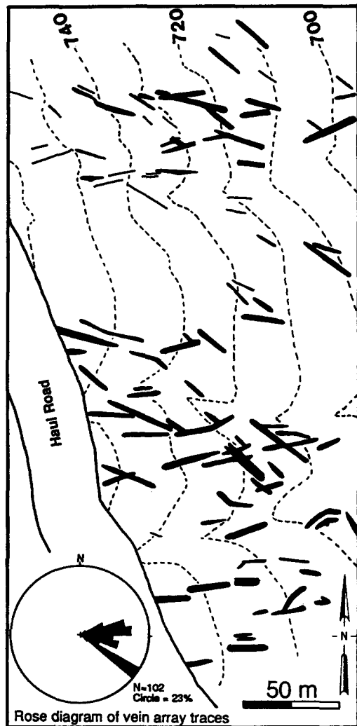
Fig. 5. Map of vein arrays and a few larger individual veins in one part of White Range mine area (contour intervals in meters; theodolite surveying and compass triangulation were used during mapping of arrays). Vein array traces shown in rose diagram. The larger vein arrays in this map area were mined along S-dipping stopes ca 1900–1910.
